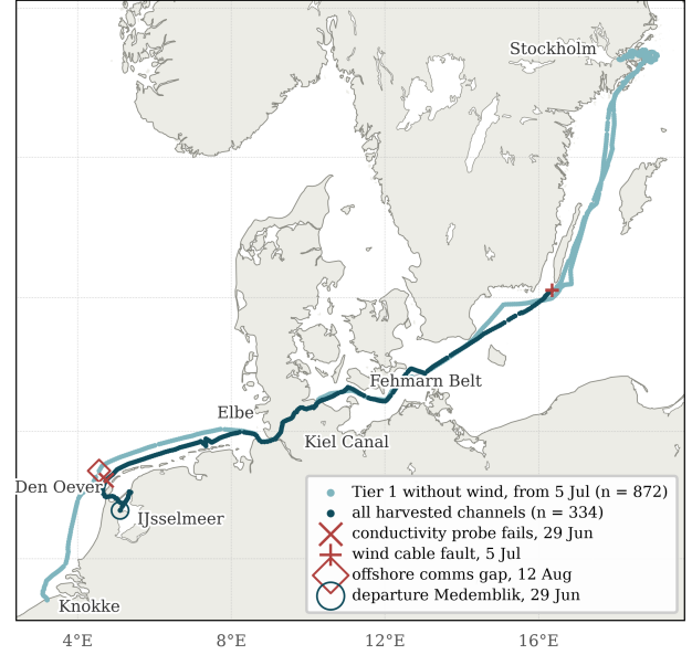
Fig. 4. Trial 3 (Medemblik, 29 June, to Knokke, 16 August 2026; n = 1,206 under-way observations), coloured by harvested-channel availability: all channels live (dark, n = 334 ) and Tier 1 without wind from the vessel’s wind-cable fault of 5 July (light). Markers: departure ( \odot ), conductivity probe failure at Den Oever ( \times ), wind-cable fault ( + ), and the offshore communications gap of 12 August that began at 8.9 kn and was backfilled on regaining the link ( \odot ). The 84 observations from the moored period (2–28 June) are not shown; statistics in the text use the 1,080 observations to 10 August. Route: IJsselmeer \rightarrow Den Oever \rightarrow German Bight \rightarrow Elbe \rightarrow Kiel Canal \rightarrow Fehmarn Belt \rightarrow open Baltic \rightarrow Stockholm archipelago, returning to Knokke.
