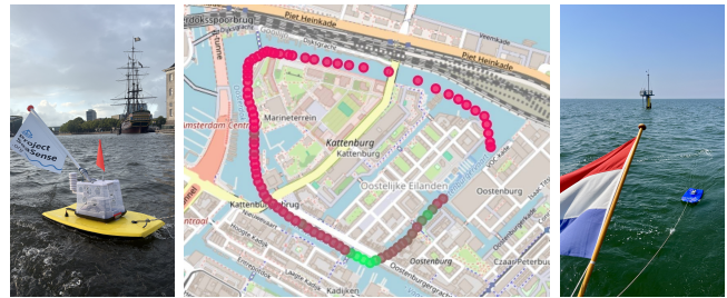
Fig. 1. Two Project SeaSense trials (cf. Section V): [left] 2025 city trial using a paddleboard, in the city of Amsterdam, with [center] showing the course taken; [right] 2026 open water deployment from a boat around a governmental measuring station.
