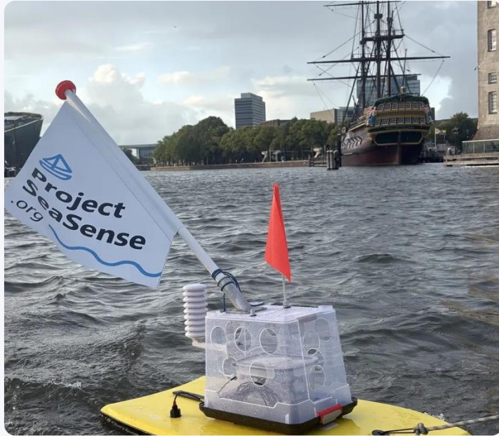
Trial 1. Sensor buoy towed behind a paddleboard through Amsterdam.
